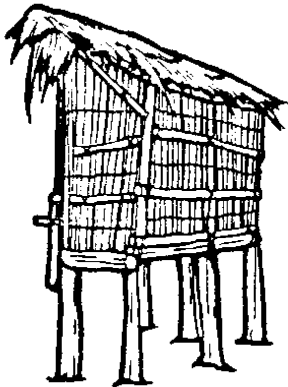
Fig. 41 Improved maize crib built from local materials
