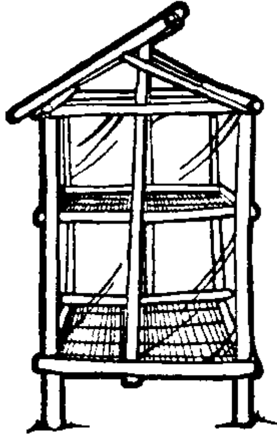
Fig. 25: Maize is stacked neatly around the perimeter, butt out, with the majority of the cobs randomly stacked inside. The roof is lifted to remove maize.
