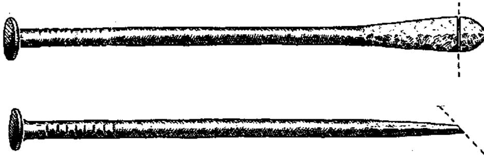
After cutting, the edge needs to be sharpened by rubbing it against a hard rock. If a hard rock cannot be found, you can buy a small file. After sharpening the edge should look like the one in the following diagram.
