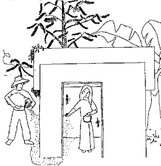
Figure 40: Site Preparation: Spreading Lime
