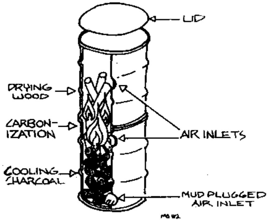
Attachment 9B: Basic principles of kiln design
